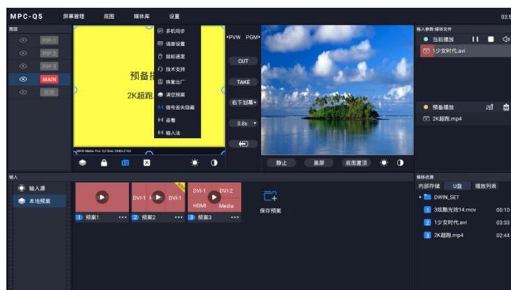
When "Plan" is selected, all the plans of the current device and the layer distribution of each plan can be viewed under the touch screen. You can call, save, update, and rename the plan in this area.
