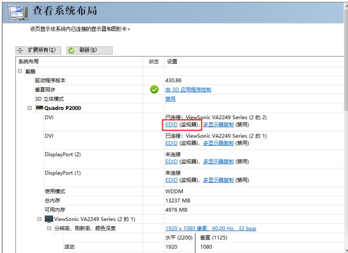
4. In the management EDID, export according to the first step of the step, select the monitor to be locked, click Export, and then generate the file as shown below to save
