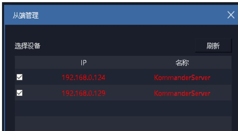
The abnormal color indicates that the connection to the slave is abnormal, causing the master to be unable to control the slave. It may be that the experimental environment of master-slave linkage has not been established, so the original white IP address and name become red. We can check the following conditions:
